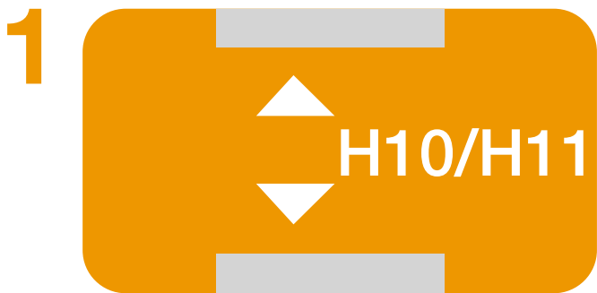
Alésage estampé grossièrement Poor tolerance of punched housing or drawn sheet metal
