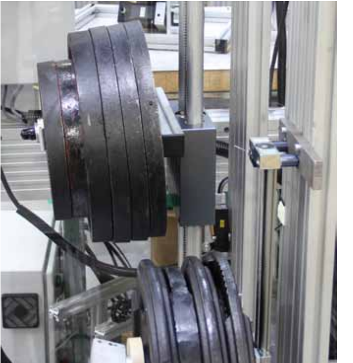
Test stand at the igus® lab to determine service life
