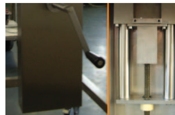
Can opener: drive for the height adjustment
